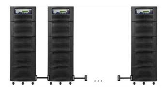
The TPH KING parallel architecture is based on a decentralized bypass architecture i.e. every UPS is provided with its own static bypass. Every UPS unit in a parallel configuration is provided with a proper output parallel Isolator which, when opened isolates the corresponding unit from the parallel system. Once the parallel isolator of a unit is open that unit is isolated from the rest of the parallel system and therefore does not provide power to the output.
